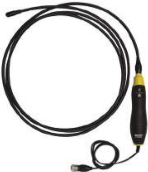
hose ø 9.00 mm, with 0° and 90° lens
