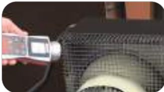
Stroboscope off: rotations not visible
