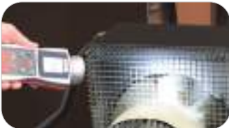
Stroboscope on: rotations visible
